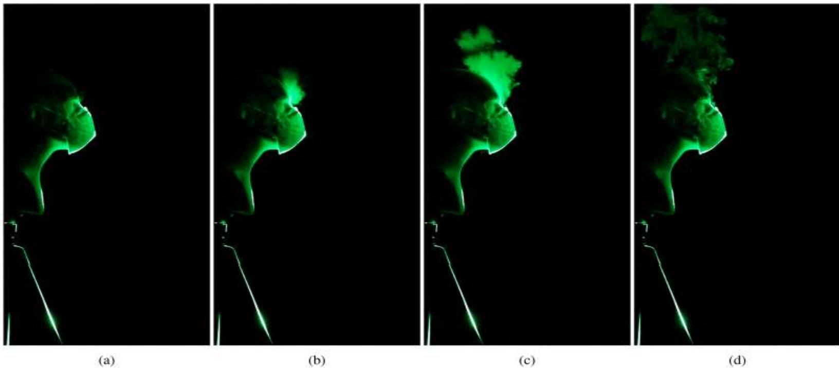
*Visualization of droplet spread when a regular N95-rated mask is used to impede the jet. (a) Prior to emulating a cough/sneeze, (b) 0.13 s after the initiation of the emulated cough, (c) after 0.33 s, and (d) after 0.83 s.*
