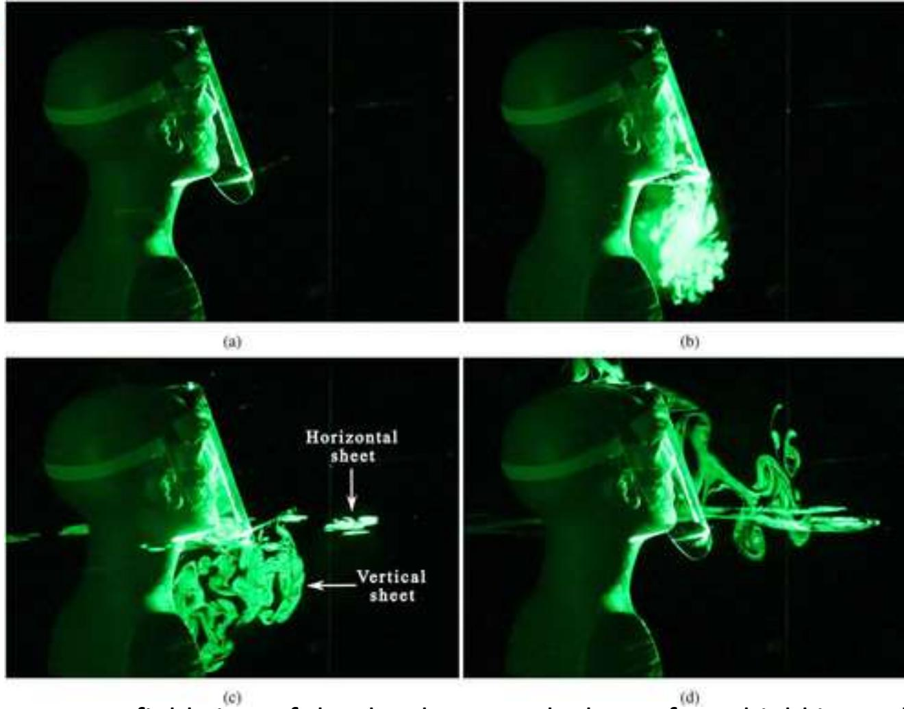
Near-field view of the droplet spread when a face shield is used to impede the emerging jet. (a) Prior to emulating a cough/sneeze, (b) 0.57 s after the initiation of the emulated cough, (c) after 3.83 s, and (d) after 16.57 s. The ejected plume is illuminated by both a vertical and a horizontal laser sheet. Droplets illuminated by the horizontal laser sheet can be observed in (c) and (d). Multimedia view: <https://doi.org/10.1063/5.0022968.1>
