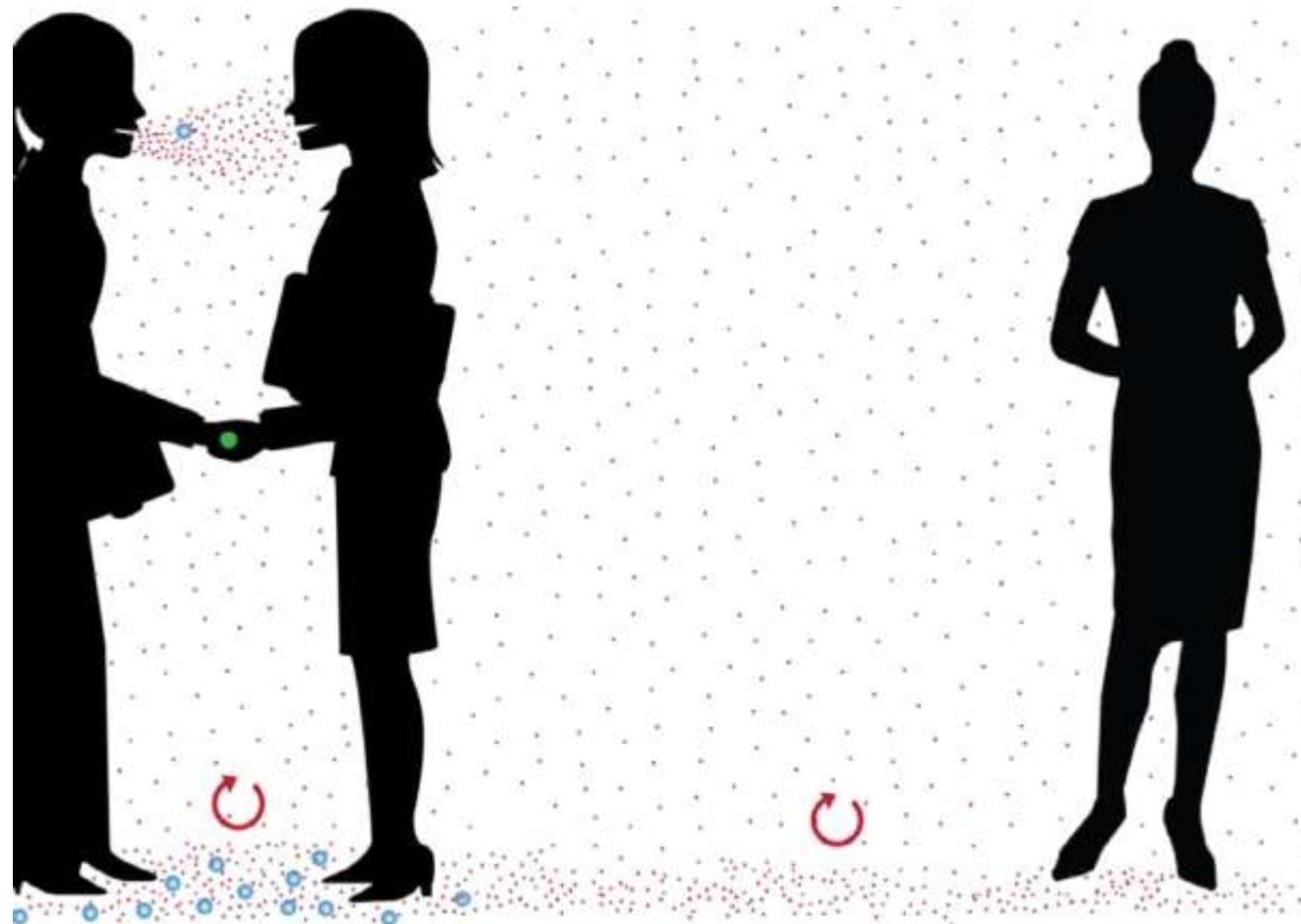
Range of respiratory particles and potential spread over distance. Blue particles represent droplets, typically  $>100$ -mm diameter, that fall to the floor under gravity within 2 m of the source. Red particles represent aerosols, typically  $<100$  mm, that stay suspended for longer, but eventually fall to the ground if the air is motionless for long enough (at least 30 min). (Tang, JHI, 2021)
